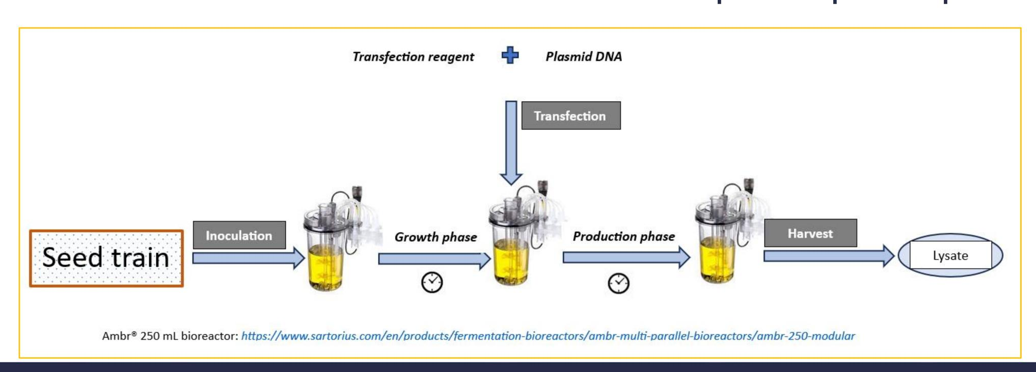
Diagram of our current upstream rAAV process platform (Ambr® 250 mL bioreactor scale).
