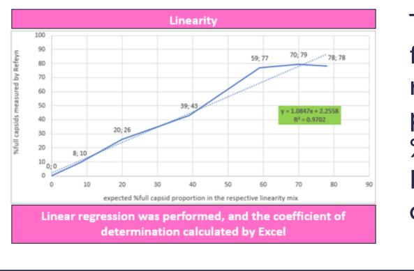
Two samples (1: 0% full; 2: 78% full) were mixed in 7 different ratios. Measured results were plotted against the theoretical %full capsids proportion. Linearity passed the acceptance criteria of  $R^2 \ge 0.90$ .
