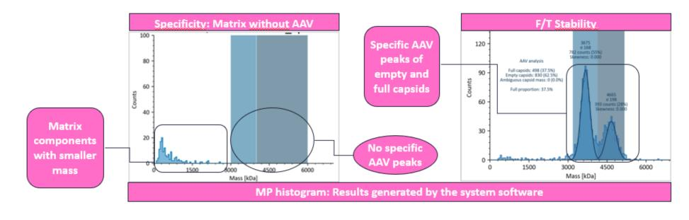
No interfering peaks were detected in the AAV-specific areas when matrix alone was measured.
